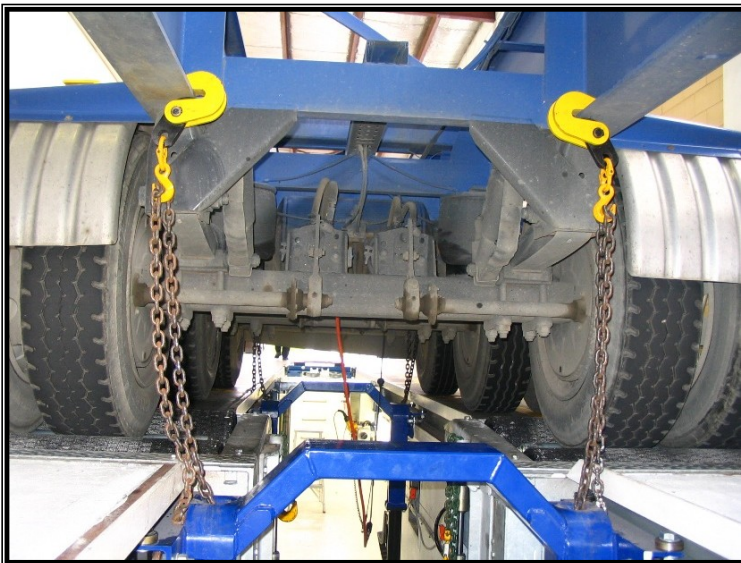
Roller brake testing of a tri-axle trailer using chassis load simulation.
